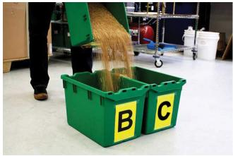
3. Pour the contents of pail A at the point where the 4. Pour the pail labelled B back into pail A. pails touch, ensuring that half the stream flows into each pail B and pail C.
