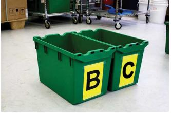
2. Place the empty pails labelled B and C side by side and touching on a level surface.
