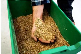
1. Place the sample you're dividing into pail A and mix thoroughly by hand.
