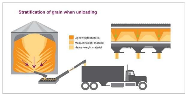
Figure 2: Stratification of grain when unloading
