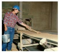
Figure 31: Sampling points for sampling grain from a horizontal belt
