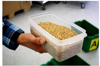
7. Place the final composite sample or samples in sealed containers and label each container to show the bin it represents.
