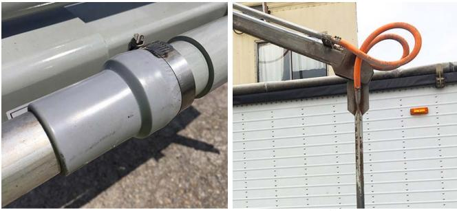
Figure 26: Rubber gasket boom sleeve
